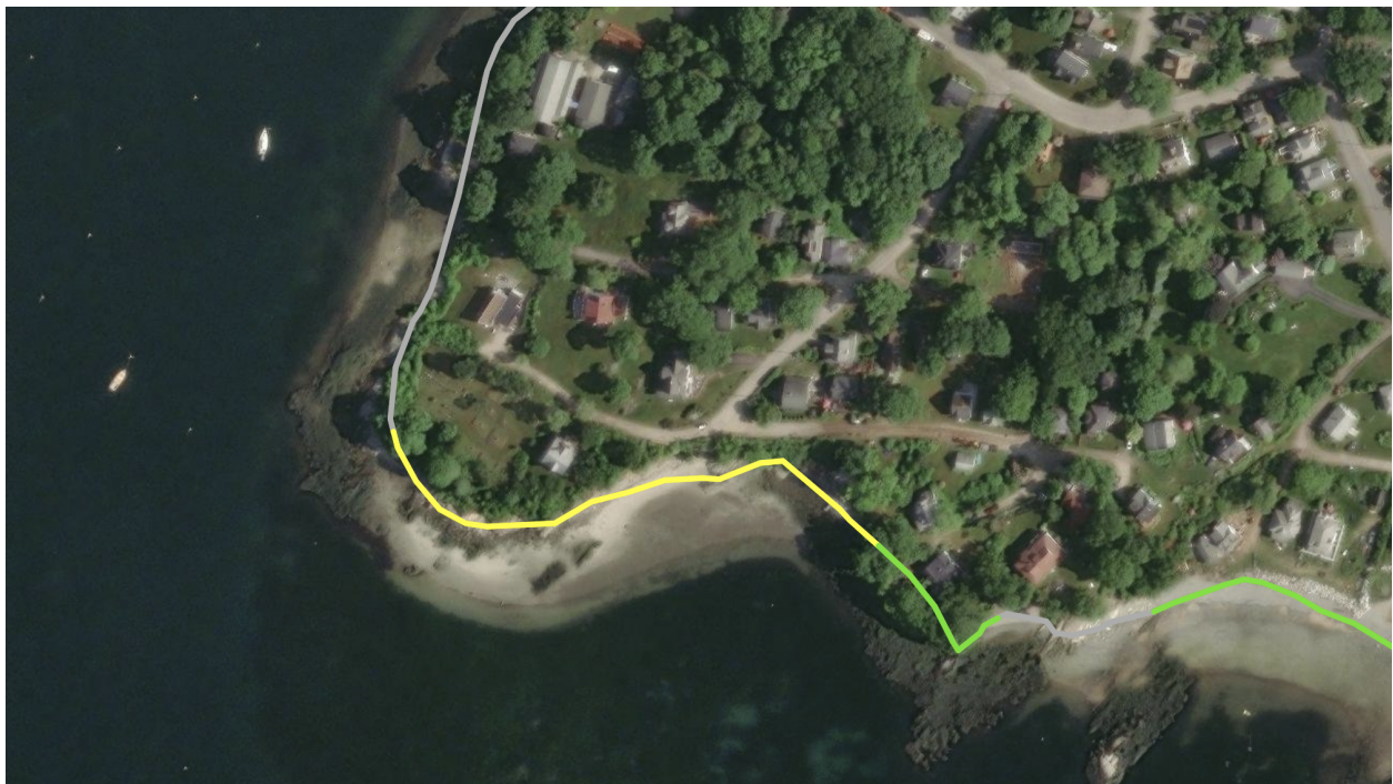
Figure 6: Coastal Bluff map of Sandy Beach from the Maine Geological Survey. The yellow line indicates areas of bluff mapped as Unstable from erosion.
