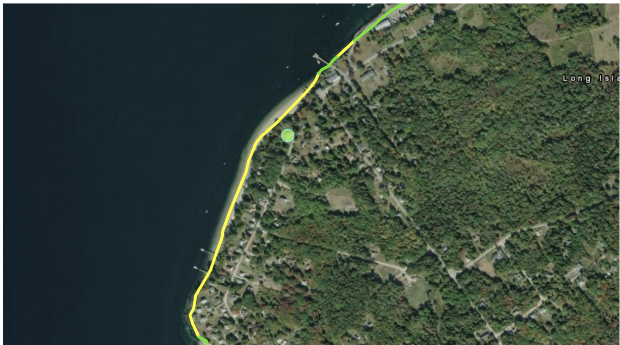
Figure 8: Maine Geological Survey Coastal Bluff map of the VFW Hall site. The yellow line indicates that the bluff was mapped as Unstable.
