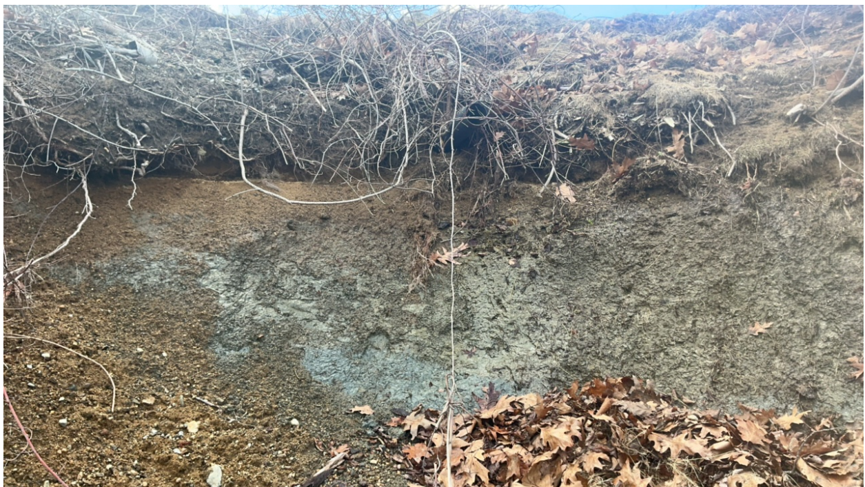
Figure 6: Dark and shimmery soil indicative of groundwater saturation near the top of the bluff face.
