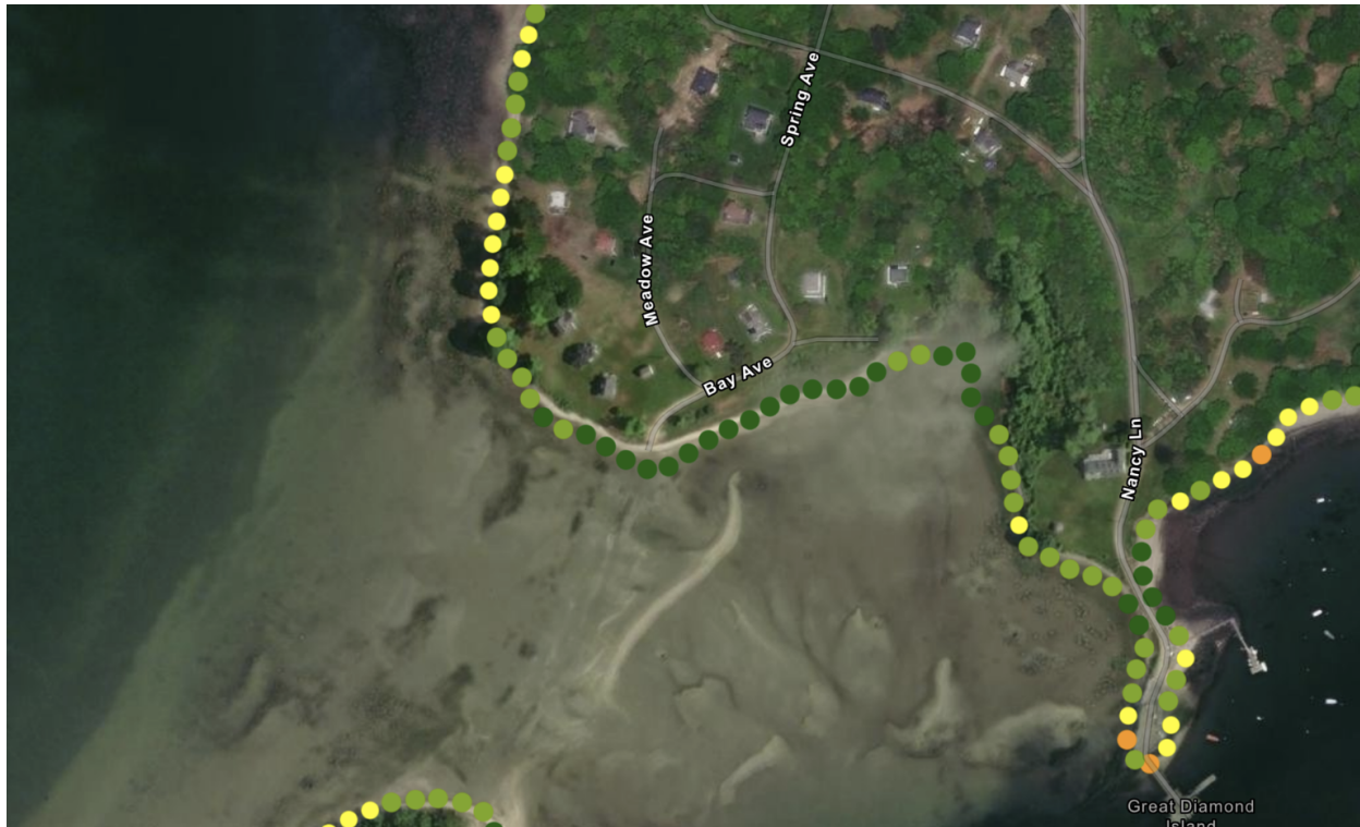
Figure 6: Maine Geological Survey Living Shoreline Decision Support Tool showing the Lamson Cove area. Dark green circles indicate that a site is ranked Highly Suitable for a living shoreline.
