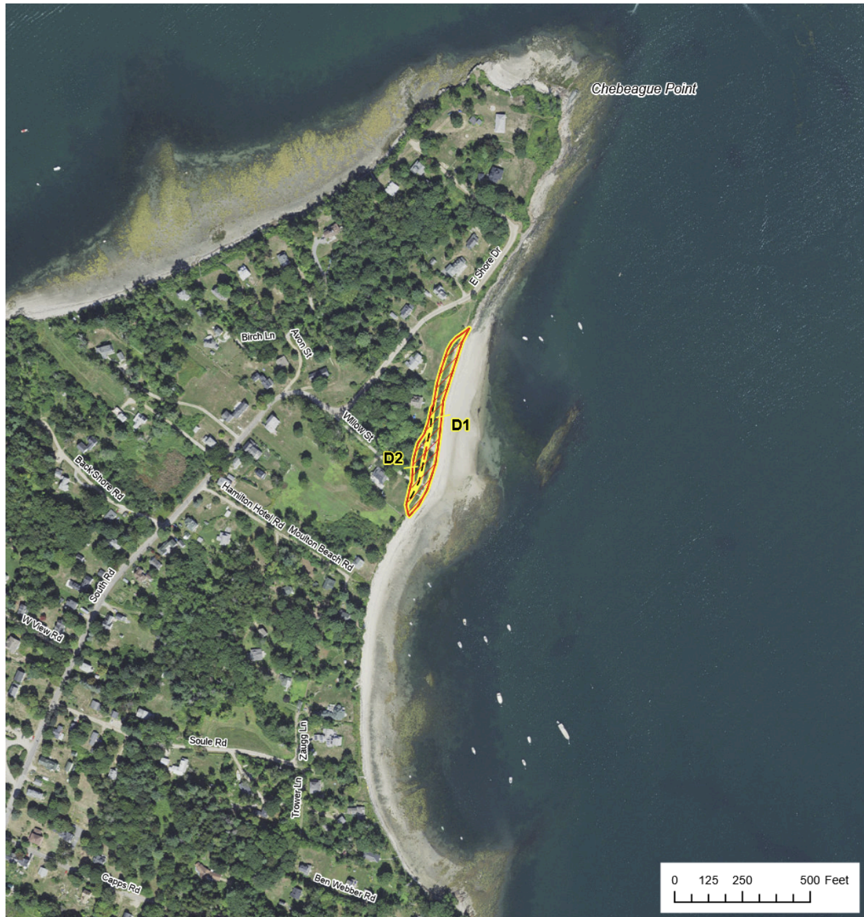
Figure 5: Coastal Sand Dune Geology of Chebeague Point including Hamilton Beach (MGS). Yellow lines delineate areas of sand dune, and red lines indicate areas at risk of erosion based on predicted sea level rise.
