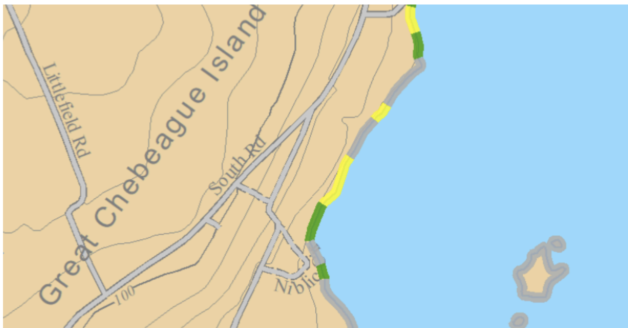
Figure 6: Maine Geological Survey Coastal Bluff Map of the assessed property and surrounding areas created in 2020. Yellow indicates Unstable bluffs and green indicates Stable bluffs.
