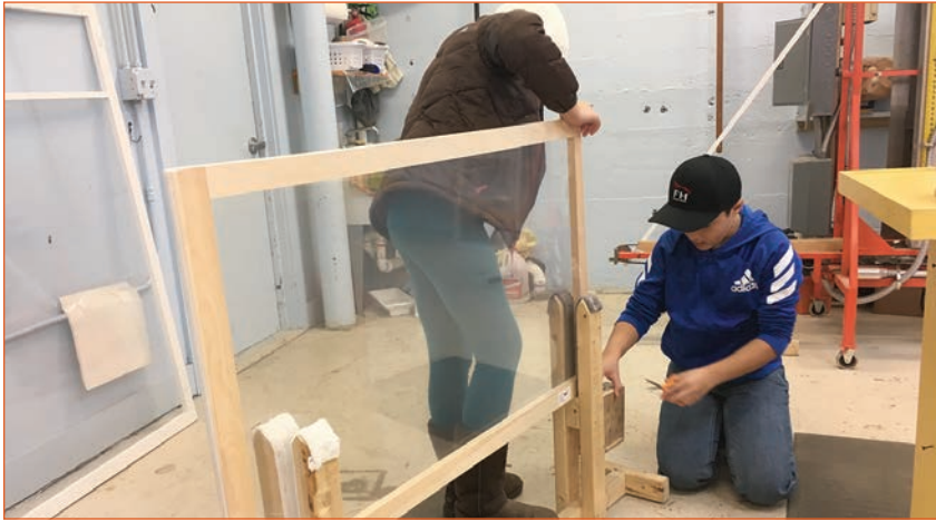
Island students build window inserts to insulate local buildings during a visit to the WindowDressers production facility.
