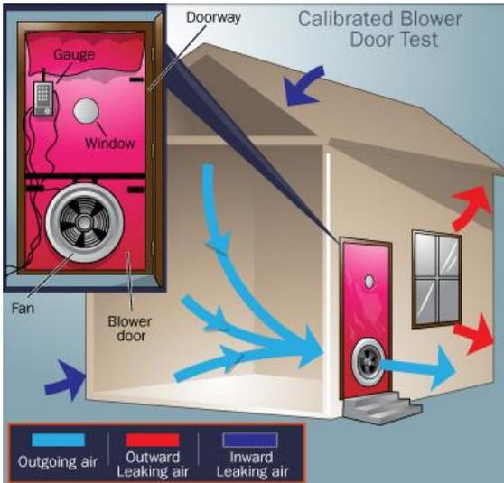
A blower door pulls air through a house, exposing air leaks. Source: How Stuff Works.
